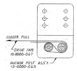
Closer with mounting tape attached under tension
